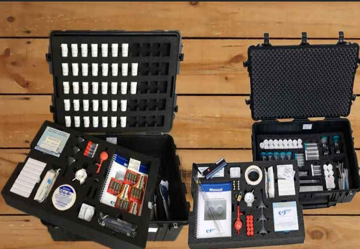
The Global Pharma Health Fund (GPHF) Minilab Test Kit
